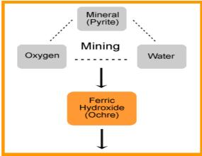
Figure 1: Mine Water Process
